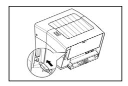
**NOTE:** Use a USB cable with a rectangular Type A plug and a square Type B plug. The USB cable should be shielded and no longer than 5 meters (16 feet) long.
